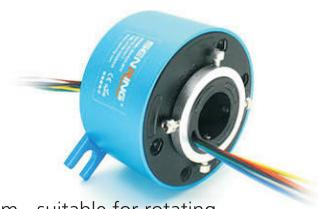
H4086 series standard precise slip ring , integrated structure design, with through hole 40mm , OD86mm , suitable for rotating application which requires a through hole <=40mm ( remark: if need a hole <40mm, can add a inner bushing)
