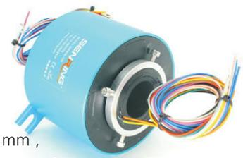
H3899 series standard precise slip ring, integrated structure design, with through hole 38.1mm , OD99mm , suitable for rotating application which requires a through hole  $\leq 38.1\text{mm}$  ( remark: if need a hole  $< 38.1\text{mm}$ , can add a inner bushing)
